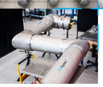
**TRANSFER LINES** are designed to transfer helium between the valveboxes. Each one includes 4 process pipes, aluminium thermal shield, DN300 vacuum envelope and vacuum barrier. Thermal compensation is realized by means of flexible hoses installed on both sides of the elbows. Total length of all transfer lines is approx. 35 m.
